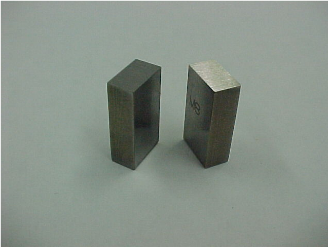
Figure 3: Photograph of blanks prior to grinding operation
